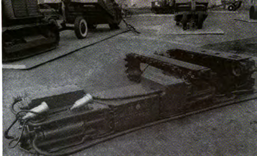
DONBAS COAL-MINING COMBINE. A model of the famous machine, pride of the Soviet mining industry, designed for gently sloping and inclined seams.
