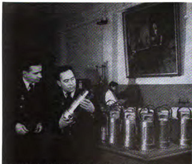
DUST METERS. By means of these instruments, the concentration of coal dust can be determined in the mine.
