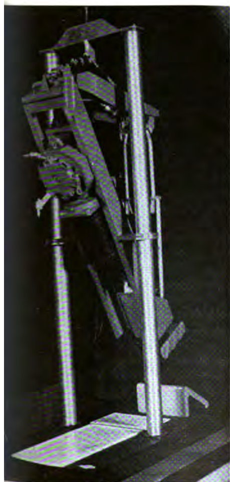
Model of the KKP-1 combine designed for working steeply sloping seams. Shown in use on preceding page.
