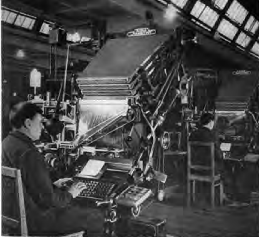
"PRAYDA" PLANT. The print shop is equipped with four-magazine machines.
