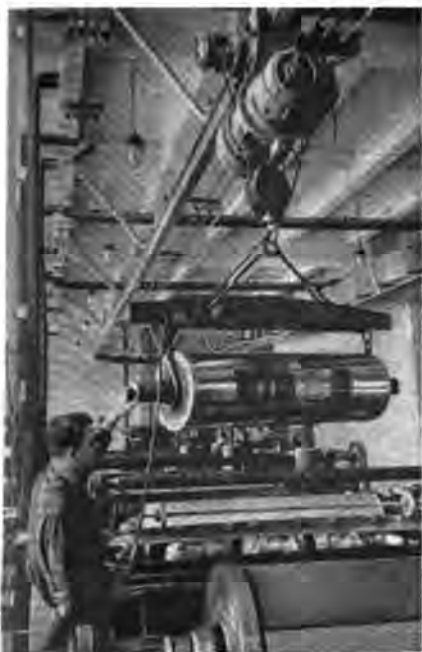
ABOVE. A worker sends a rotogravure cylinder form to the presses by means of an overhead conveyor.
