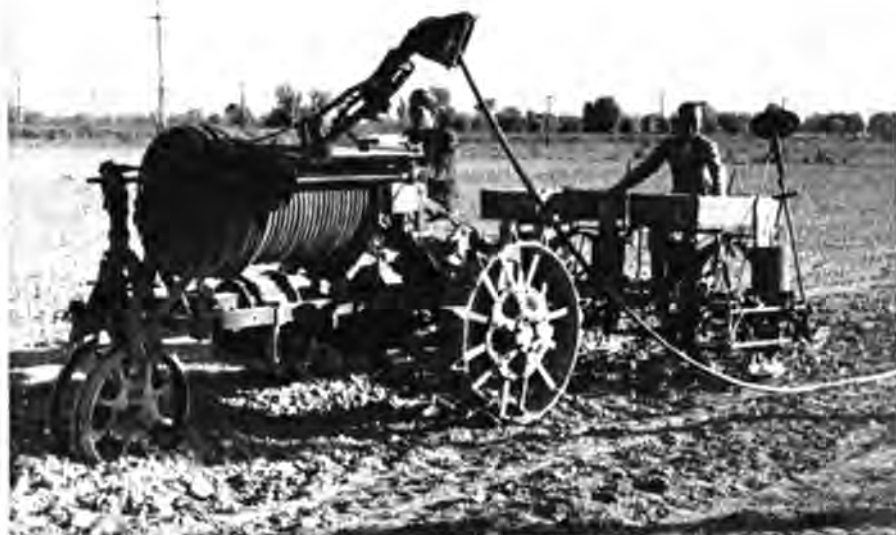
ELECTRIC TRACTOR. Tractors powered by local electricity are used on many Uzbek collective farms. This one is working the fields of the Communist Collective Farm.
