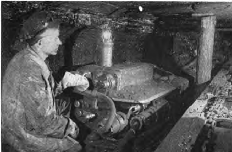
MECHANIZATION. Electric mining combines like this one cut, strip, and load coal, thus eliminating arduous work. Soviet mines are the world's most mechanized.
