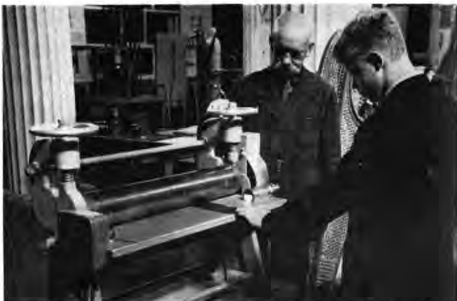
PHOTO-ELECTRIC EYE. This cell on a sheet rolling machine stops the motor if the operator's hands get too close. The automatic shut-off protects the worker from industrial accidents.
