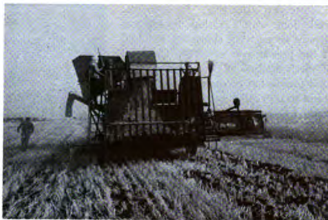
MECHANIZED OPERATIONS. A tractor-drawn cultivator (left) on a field of sugar-beet, also planted by machine in a carefully spaced geometric pattern. A self-propelled combine (right) on a Kuban farm, fitted with special devices for stacking straw and chaff.
