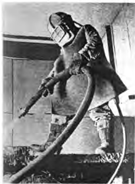
SAFETY SUIT. Used by workers cleaning metal castings at the Urals Machine Building Plant.
