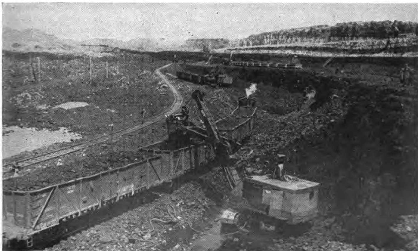
KARAGANDA COAL FIELDS. The open-cut method is used. An excavator loading coal into the cars.
