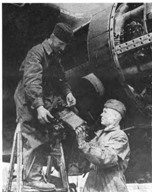
Electricians install a new generator
