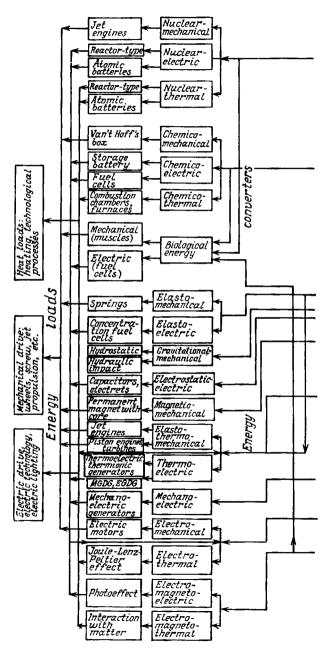
Flow Diagram of energy Sources, Conver (read the diagram
