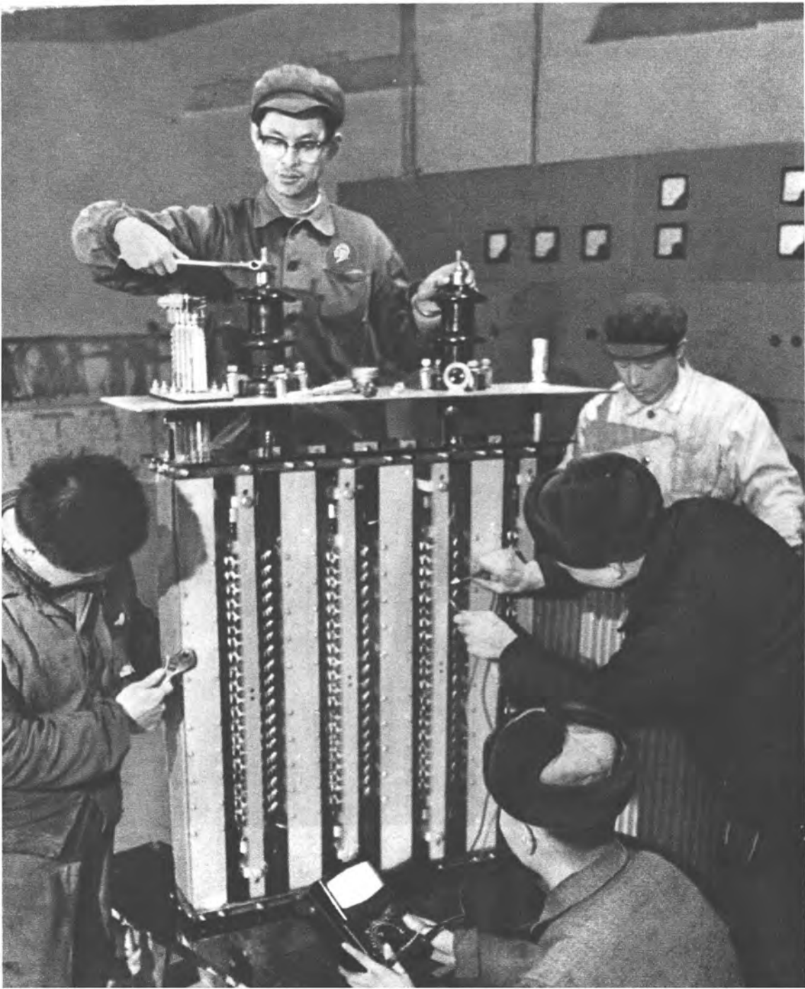
After having succeeded in creating a disk type silicon power diode up to the advanced level of the 60's, the revolutionary workers and staff members of the Peking Transformer Factory successfully produced a high power silicon rectifier unit.
