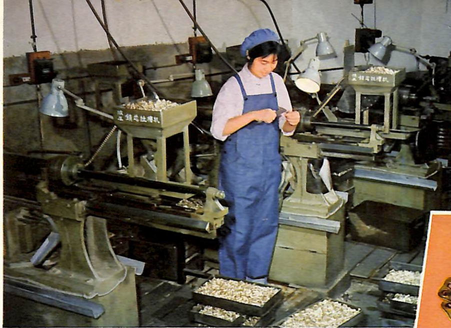
Hydraulic machine for groove cutting of lock cylinders.
