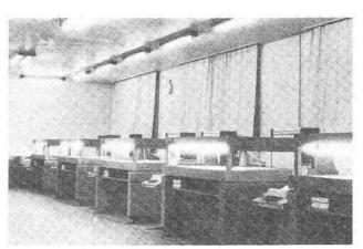
The X-Y plotting machines automatically plot synoptic charts for forecasting.
